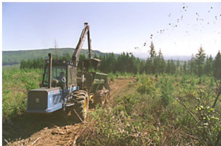
King County, Seattle, WA, Application of Dewatered Biosolids with Flinger in Forest Areas
