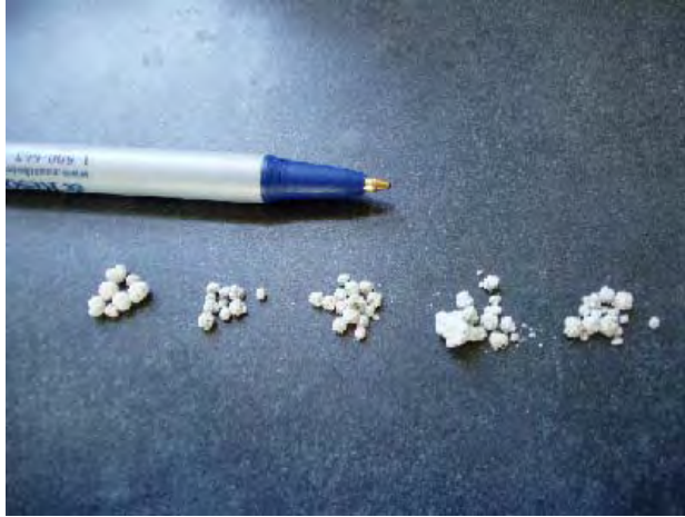
Figure 2: Struvite Crystals Formed During Pilot Study
