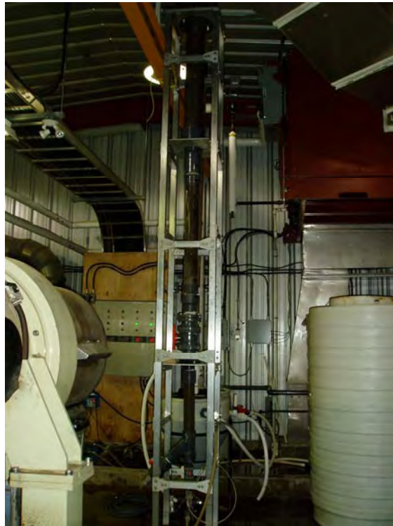
Figure 1: Crystallizer UBC Pilot Assembly
